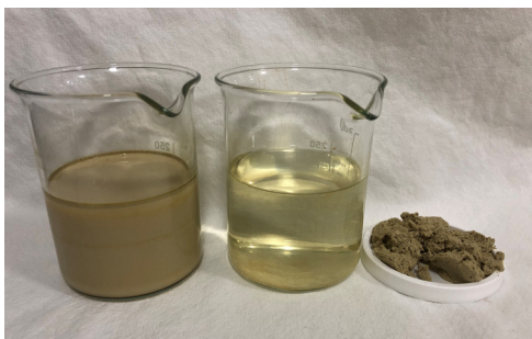
To the left the wastewater to be purified. The AxoPur process separates the wastewater into purified water (center) and a floc (right).
